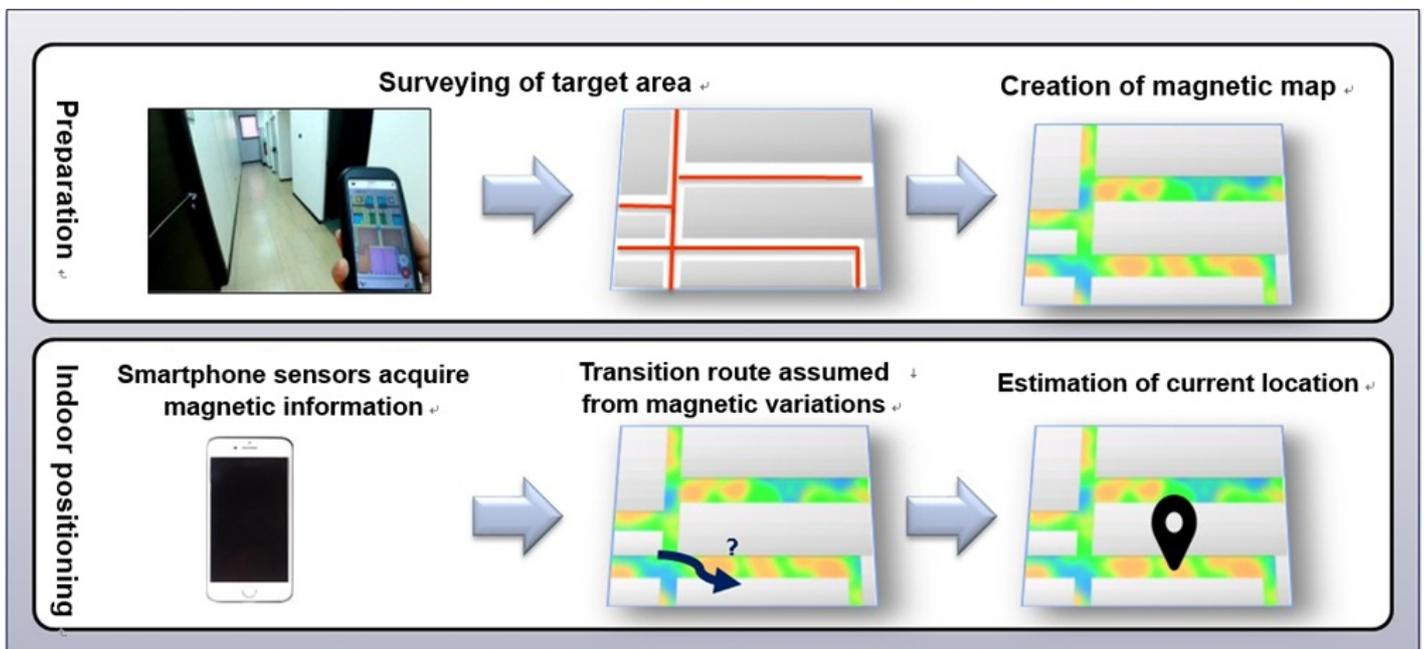
Figure 2: Structure of indoor localization through geomagnetism
